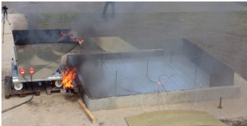
Figure 15. All visible flames disappeared approximately 6 seconds after tipping the burning oil into the pit.
