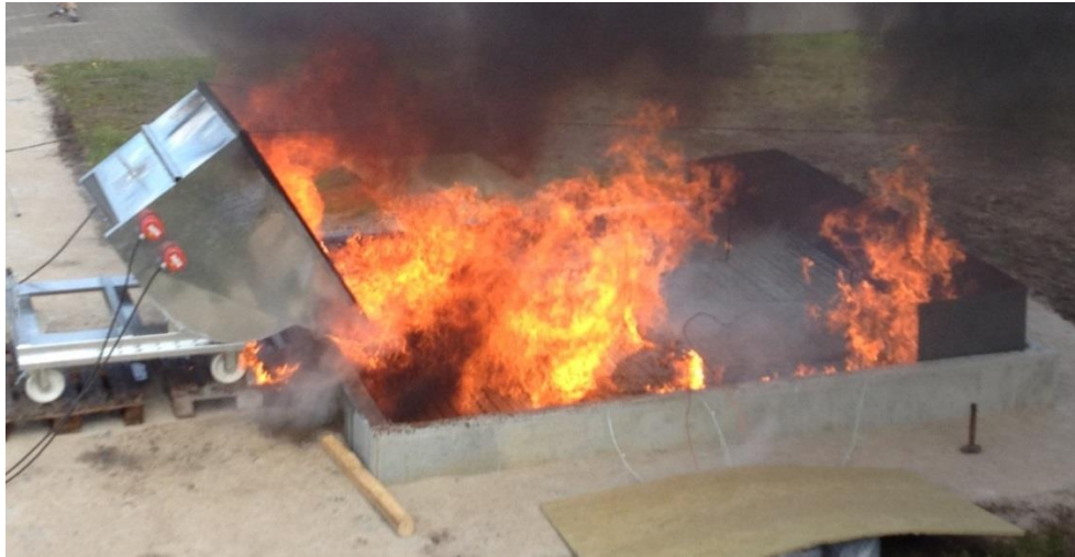
Figure 14. Flames were visibly smaller within a few seconds after tipping the burning oil into the pit.
