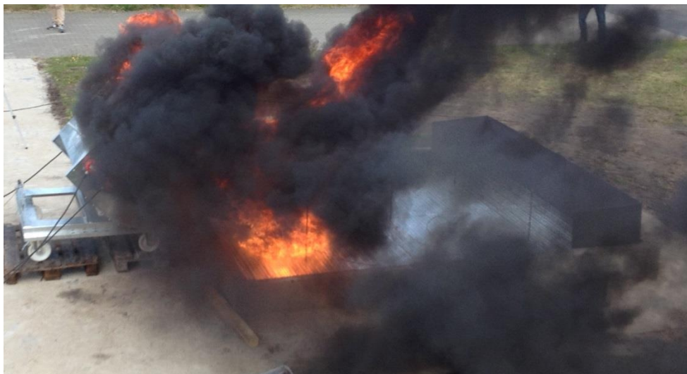
Figure 12. Tipping the burning oil into the pit.
