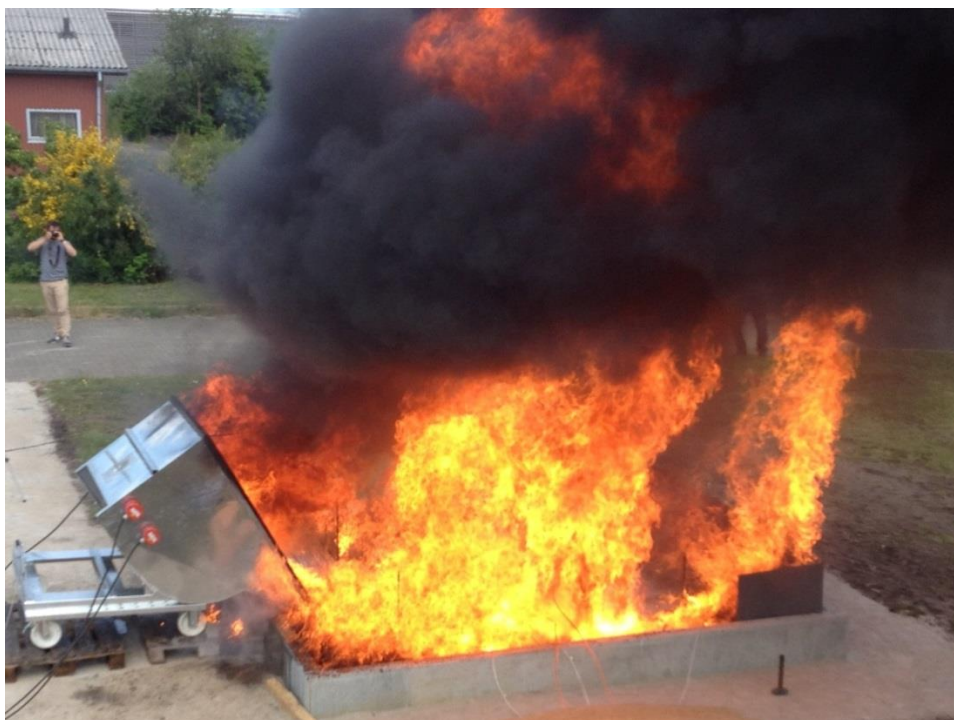
Figure 13. High intensity of the flames after tipping the burning oil into the pit.
